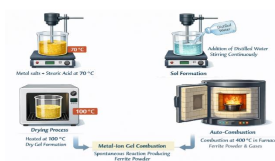
Figure 1. Synthesis procedure of Ni_{1-x}Mn_xFe_2O_4 ferrite powders
