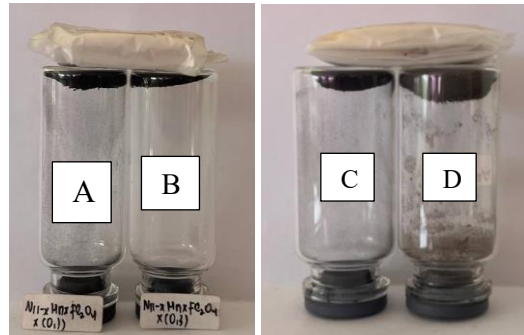
Figure 3. Ni_{1-x}Mn_xFe_2O_4 Magnetic Attraction Test Results A. x(0,1) , B. x(0,3) , C. x(0,7) , and D. x(0,9)
